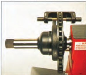
5. DISC STABILIZER. A West exclusive. The finest vibration dampener on the market is standard equipment. Rotor setup is fast and easy. No need to spend time installing rubber silencer bands.
