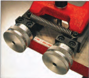
7. DEPTH OF CUT is simple to set using adjustable “zero” feature on knobs and handwheels. Graduations are shown in millimeters and inches.
