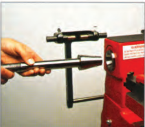
9. REMOVABLE ARBOR allows for quick and easy changeover to mount specialized adaptors for truck, foreign cars or flywheels.
